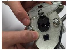
3. On the locking mechanism there is an arm to indicate how far to push the tube through
