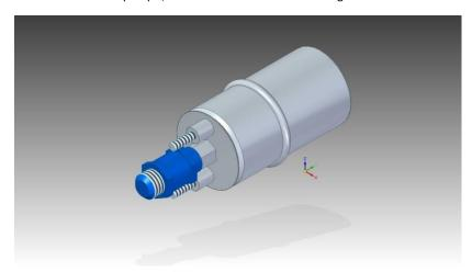
II. Fit the pump retaining bracket and bolt to the spacer using the supplied M6 18mm UHL cap screw. Use the 3 remaining M6 18mm UHL cap screws to secure the pumps.
