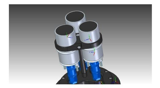
**III. NOTE:** If you are using only one or two pumps, replace the swivel fitting with a -8ORB port plug (Not supplied with kit) Fit the check valves to the fuel pump inlets.
