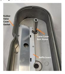
9. Install the new valve cover bolt sleeves by carefully working the new grommets into the valve covers until they are fully seated into each opening.
