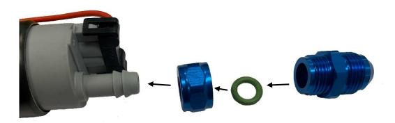
2. Lube up the O-ring thoroughly with an appropriate lubricant. Carefully not to tear, slide the O-ring over the barb's edges. The O-ring must seat against the lowest barb edge.
