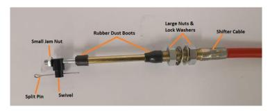
5. Move the transmission Chrysler selector lever by hand all the way to the rear position (Low Gear). Shift the shifter assembly to the Low Gear position. Adjust the large nuts on the cable so that the swivel will slide into the hole on the selector lever. Tighten the large nuts completely. Be sure that the swivel will slide freely in and out of the hole in the selector lever.
