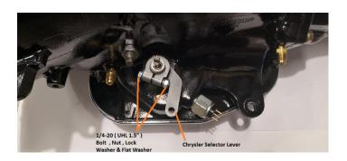
2. Remove the two transmission oil pan bolts directly below the shifter lever. Install the Chrysler cable bracket into position with two spacers between the pan and the bracket. (If your transmission is equipped with a cast aluminium oil pan these spacers do not have to be used). Install the two supplied 5/16-18" (UHL 1.00") bolts and tighten to 12-13 ft. lbs (16-17 Nm). Do not overtighten as this can damage the transmission pan gasket.
