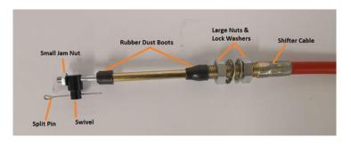
7. Move the transmission Ford selector lever by hand all the way to the rear position (Low Gear). Shift the shifter assembly to the Low Gear position. Adjust the large nuts on the cable so that the swivel will slide into the hole on the selector lever. Tighten the large nuts completely. Be sure that the swivel will slide freely in and out of the hole in the selector lever.
