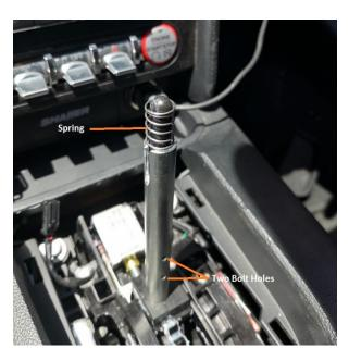
**4.** Before placing the shifter assembly onto the stick. Place the provided spring on top of the stick like shown.
