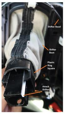
2. Now you can start to install the Attack shifter. Push the Attack shifter handle through the OEM shifter boot. By orienting it correctly with the machined groves and the lever should be facing the front of the shifter bezel assembly. Ensure the Attack shifter is pushed all the into plastic ring square. You can do this by placing the billet spacer mount over the top and ensuring the holes line up correctly.
