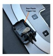
3. Using your Phillips head screwdriver, remove the inner screw from inside the cavity in which the rear plastic trigger cap was removed.
