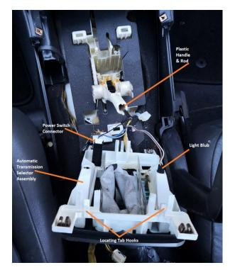
17. Remove the automatic transmission selector assembly from the vehicle and place on workbench.
