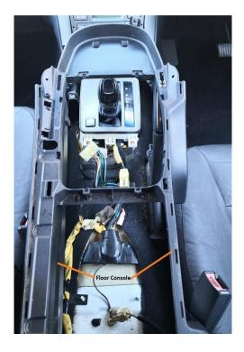
**14.** Remove the one torx bit screw located behind the OEM shifter handle. Ensure to keep this screw as it will be reused for the installation late on.
