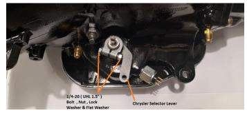
2. Remove the two transmission oil pan bolts directly below the shifter lever. Install the Chrysler cable bracket into position with two spacers between the pan and the bracket. (If your transmission is equipped with a cast aluminium oil pan these spacers do not have to be used). Install two 5/16-18" ( UHL 1.00" ) bolts and tighten to 12-13 ft. lbs ( 16-17 Nm ). Do not overtighten as this can damage the transmission pan gasket.
