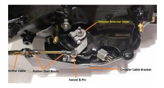
If you have a problem, DO NOT FORCE THE SHIFTER, this will damage the cable, the shifter or the transmission. Simply start at the beginning and carefully check all your steps.
