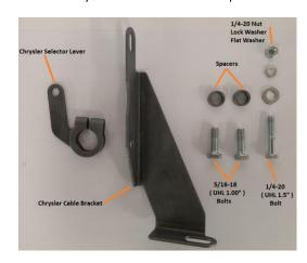
2. Remove the two transmission oil pan bolts directly below the shifter lever. Install the Chrysler cable bracket into position with two spacers between the pan and the bracket. (If your transmission is equipped with a cast aluminium oil pan these spacers do not have to be used). Install the two supplied 5/16-18" (UHL 1.00") bolts and tighten to 12-13 ft. lbs (16-17 Nm). Do not overtighten as this can damage the transmission pan gasket.
