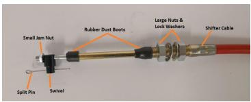
9. Thread the swivel & pin onto the cable to about the middle of the threaded section, then reinstall, but do not tighten the jam nut at this stage. Before proceeding, verify that forward gear selector pin and C-Clips are installed in the correct position that is required for
