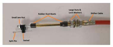
5. Move the transmission Chrysler selector lever by hand all the way to the front position (Low Gear). Shift the shifter assembly to the Low Gear position. Adjust the large nuts on the cable so that the swivel will slide into the hole on the selector lever. Tighten the large nuts completely. Be sure that the swivel will slide freely in and out of the hole in the selector lever.
