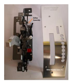
8. Now the shifter assembly is bare. To reinstall the billet cover, follow the steps in reverse.
