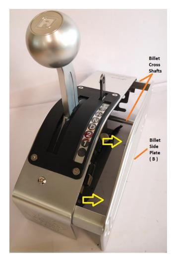
5. Unscrew the billet round gear knob from the shifter handle.
