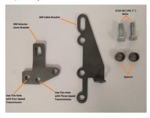
3. Install the selector lever bracket using the stock selector lever nut, and tighten the nut to 23 ft-lbs (30 Nm) torque. The lever should travel smoothly back and forth, with a positive "click" in each detent.
