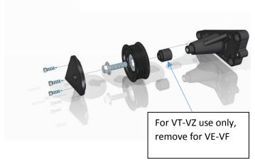
Designed to work with both VT-VZ (Pontiac GTO) and VE-VF (Pontiac G8 & Chevy SS) belt lines this power steering delete kit replaces the power steering pump on non-power steering vehicles and vehicles with electric steering and/or steering pumps. Use as pictured for VT-VZ belt line, for VE-VF remove the spacer between the pulley and the main body.
