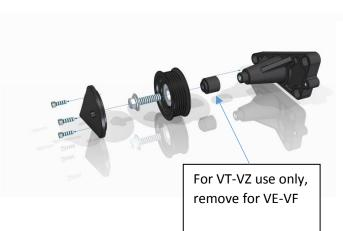
Designed to work with both VT-VZ (Pontiac GTO) and VE-VF (Pontiac G8 & Chevy SS) belt lines this power steering delete kit replaces the power steering pump on non-power steering vehicles and vehicles with electric steering and/or steering pumps. Use as pictured for VT-VZ belt line, for VE-VF remove the spacer between the pulley and the main body.
