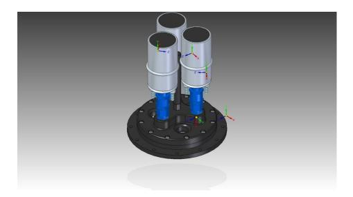
Fit the pump retaining bracket and bolt to the spacer using the supplied M6 18mm UHL cap screw. Use the 3 remaining M6 18mm UHL cap screws to secure the pumps.
