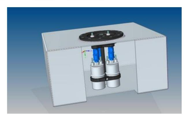
The Aeroflow Triple Pump in-tank is designed to work with up to 3 Aeroflow AF49-1013 in-tank fuel pumps in an aluminium tank that is 250mm deep. If using with less than 3 pumps additional fittings will be required to block the un-used inlets.
