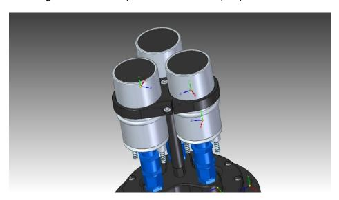
Connect the wiring to the first pump and using the supplied short wires connect the first pump to the second and third pumps. If you're unsure of the correct way to wire the pumps please consult an auto electrician.
