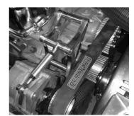
Shown fitted along with an Aeroflow AF64-3003 gilmer drive kit and matching AF65-1006 belt
