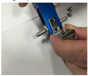
3. Once all adjustment are completed tighten the detent screw to fix in the final position.
