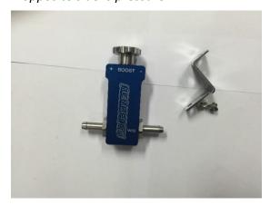
2. The boost tee should always be fitted with the boost pressure backed off by winding the knob counter clockwise then slowly increased until you reach your desired boost pressure.
