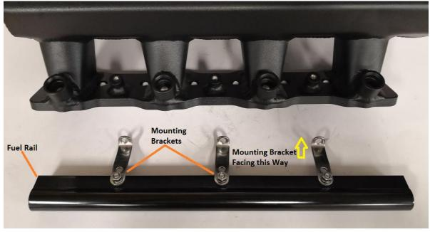
2. Apply a silicone lubricant to the O-ring on the inlet end of the factory OE fuel injector (sold separately) and insert the fuel injectors into the ports in the fuel rail. To insert the injector without tearing the O-ring, gently rock the injector in the inlet of the port while applying pressure to insert the injector.
