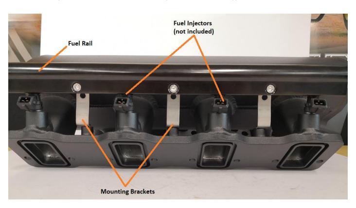
5. Tighten the fasteners in two steps – 3.6 ft-lbs (5 Nm) and then to 7.41 ft-lbs (10Nm). Evenly tighten down fuel rail screws and ensure the fuel rail does not kink as this can cause the injector O-rings to pinch and leak when damaged.
