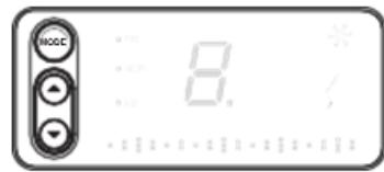
To turn off the ANTI-THEFT function, start the engine. Long press the MODE button for 2 seconds until the display light is back on.
