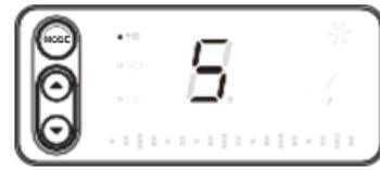
To turn off the DRAG RACING mode, simply just hit the MODE button to exit out back into the mode you had on chosen previously.
