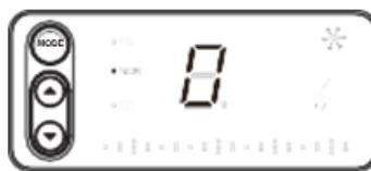
To turn off the ANTI-SLIP function, simply just hit the MODE button to exit out back into the mode you had on chosen previously.
