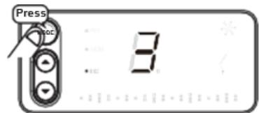
3. It will enter anti-theft mode when the display light is off. During this mode the accelerator pedal will not respond and the vehicle will not be able to be driven.
