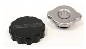
First identify what size radiator cap you have, There are two main sizes typically found world wide small size is 32mm O.D. and large size is 42mm O.D. Note: O.D. measurment excludes the ears.
