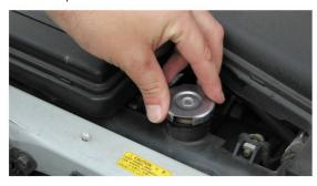
5. Fit the cap to the radiator and tighten.
