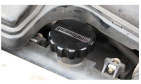
8. After allowing sufficient time for the silicon to dry, Remove the radiator cap and check to make sure the cap has been fitted deep enough into the cover. Check coolant level is correct, Re-Fit Radiator cap and Happy Motoring!!
