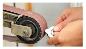
Remove the ears from each side of the cap as shown. WEAR SAFETY GLASSES!
