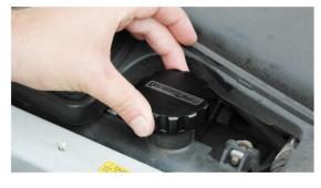
Fit the Aeroflow Radiator cap cover in the position you desire and press firmly, being careful not to damage the radiator
