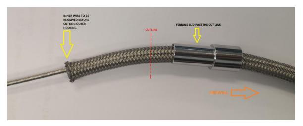
6. To cut the throttle cable measure the distance between the throttle cable adjuster and the firewall fitting. Add 2" (50.4mm) to the measurement and mark a cut line on the cable housing at that length.
