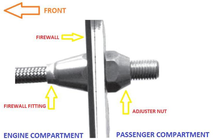
2. From the engine end of the Aeroflow throttle cable, remove the throttle cable adjuster and the carb end assembly. If the cable housing is braided stainless steel, DO NOT REMOVE the ferrule. Pull the inner wire out of the cable housing.
