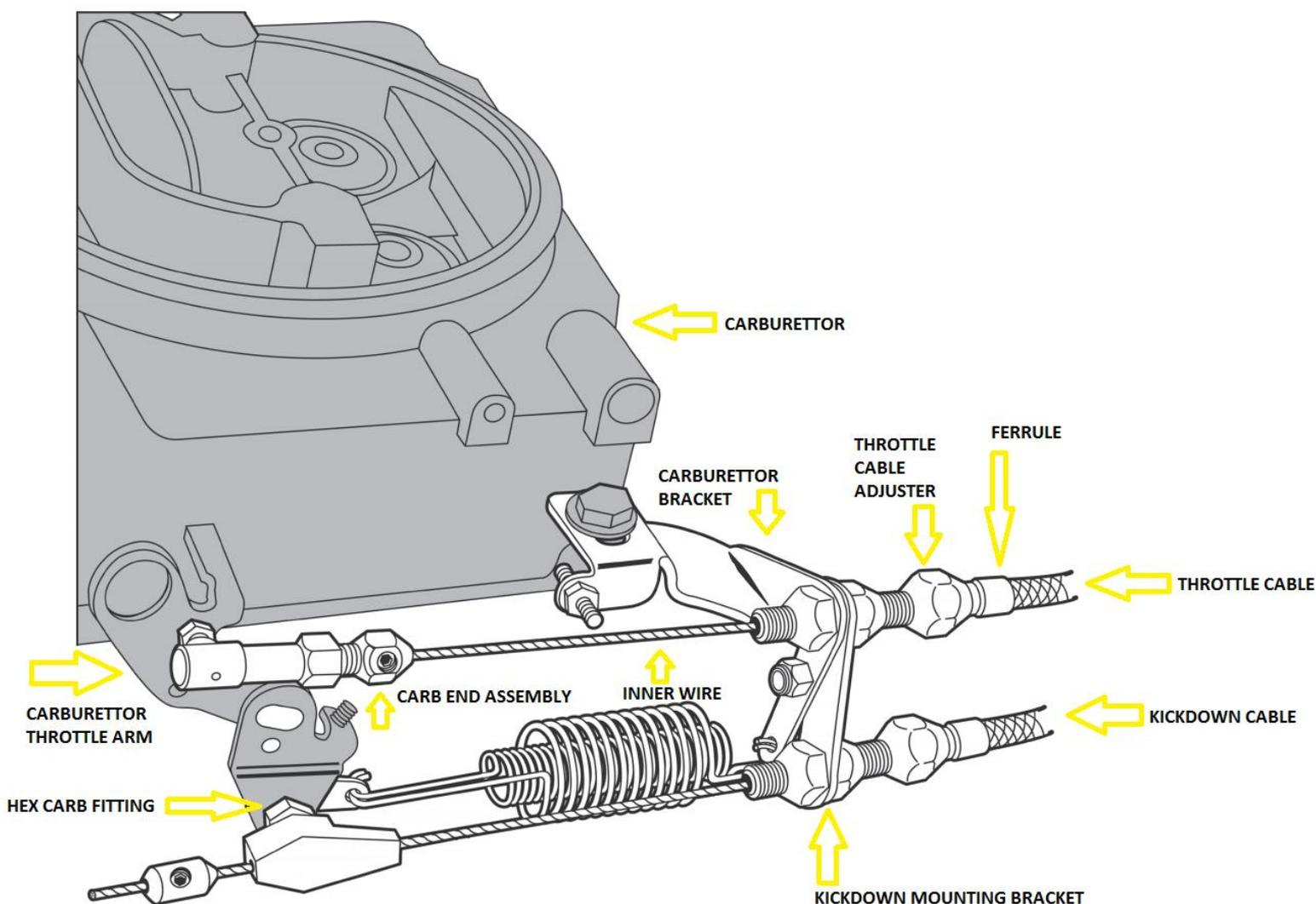
Throttle Cable shown with Aeroflow Carburettor Bracket and Springs AF42-1104 and Kickdown Kit ( Sold Separately )
