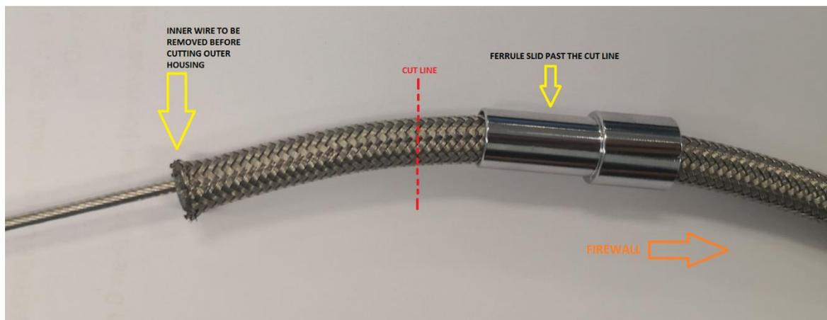
6. Reinstall the inner wire into the cable housing from inside the passenger compartment. Ensure that you connect the clevis (or the ball end if the clevis has been removed) on the new Aeroflow throttle cable to the throttle pedal.
