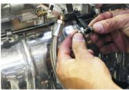
14. Once your happy with the position bolt the arm to the accelerator linkage arm using small brass bush in between rose joint and arm. Make sure to use the long cap screws supplied.
