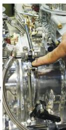
15. Check that you are getting full throttle and that the linkages are not binding or interfering with anything. Move the arms sideways on the spline to get the linkages working as straight as possible.
