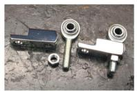
4. Install rose joints into carburettor blocks.
