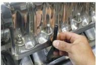
5. Install supplied extended studs to blower manifold where the accelerator plate will mount.
