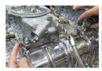
7. Mount the carburettor blocks onto the carburettor studs. Make sure the rose joint is facing down
