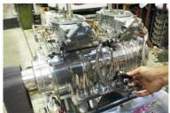
19. Check all cap screws and nuts are tight and that the linkage works freely and doesn't bind. Make sure both carburettor arms pivot at the same angle and trigger both carburettors simultaneously. Make sure you have full throttle and return to idle.
