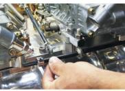
11. Feed long splined shaft through rose joint, 12. Install arm onto splined shaft at long keep the short section of spine at the front. Fit one of the billet stoppers, make sure to loosen grub screw on stopper. Then feed the shaft through the front rose joint.
