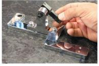
2. Attach the arm to one side of the short shaft 3. Attach another arm to the other side at and feed through roller bearing. Should be a nice fit and swing easily with no slop.
