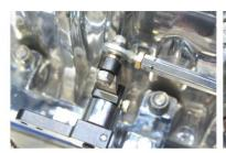
10. Install adjustable linkage arm to accelerator arm, use small brass bush in between rose joint and arm. Make sure to use the long cap screws supplied.
