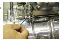
17. Install the other brass stopper at the front of the splined shaft and tighten grub screws on both stoppers.
