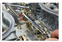
9. Install adjustable linkage arm to carburettor next to brass bushes with nyloc nut. Make sure to use the long cap screws supplied.
