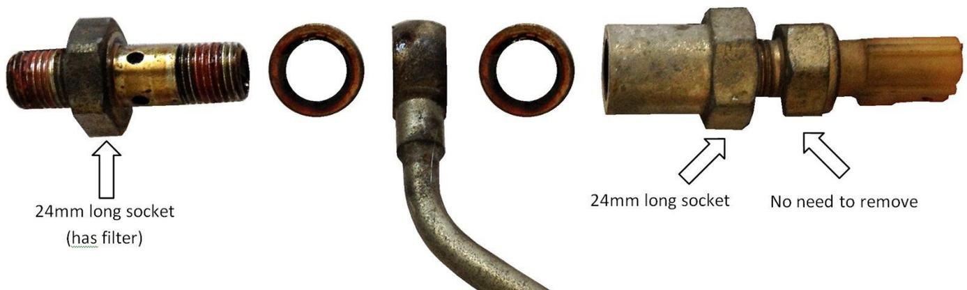
2. Install 7/16 fitting into top of turbo
